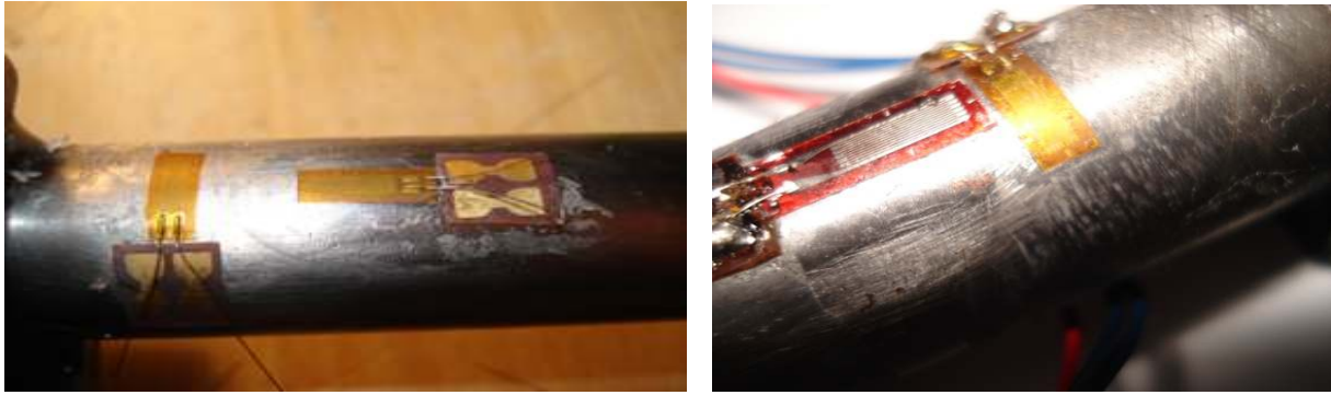
Figure 6.29 Mounted Load Cell Arrangement - B.Hand 2014
