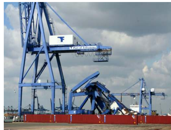
Figure 3.13 Crane Failure due to Wind-Induced Loading [19]
