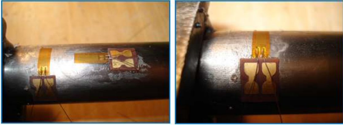
Figure D7 Orientation of Strain Gauges for prototype testing B.Hand 2014
