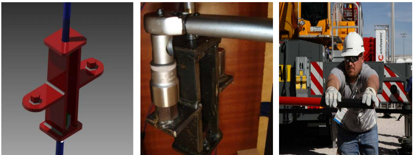
Figure 6.11 Effective generation of tensile loads via effective torque setting – B.Hand 2014
