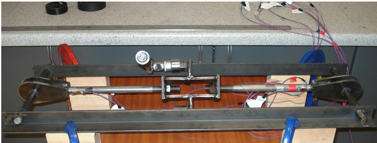
Figure 6.30 Experimental Test Rig Torque Application and Force Measurement Configuration - B.Hand 2014
