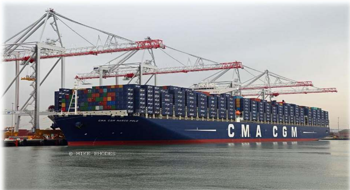
Figure 8.1 Liebherr Super Post-Panamax STS Container Cranes Operating at Port of Southampton, United Kingdom [1]
